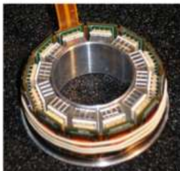
Fig. 1. The RatCAP tomograph consisting of 12 LSO arrays with APDs and associated readout electronics.
