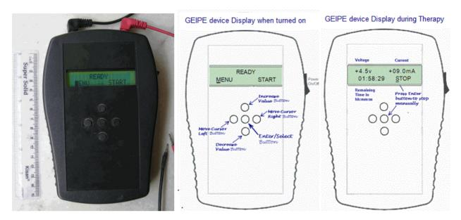
The latest GEIPE device, built in early 2010, is based on solid-state electronics and can provide DC electricity for the GEIPE therapy in either constant current or constant voltage mode. It runs on four AA batteries – preferably rechargeable.
