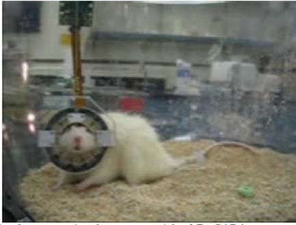
Fig. 5. Awake rat wearing the RatCAP that is supported by the tether and mechanical counterbalance system.
